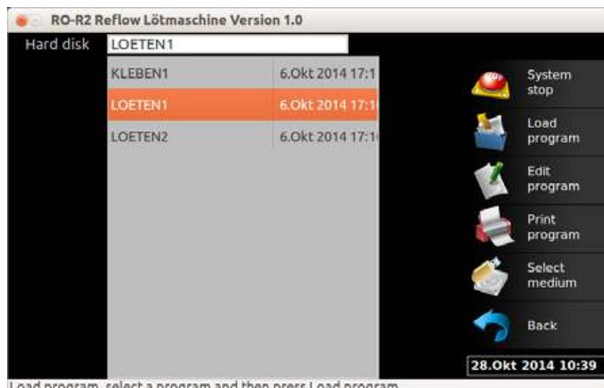
A file window opens showing all solder programs stored on the hard disk. In case that you want to load solder programs from a USB mass storage or network (option):
