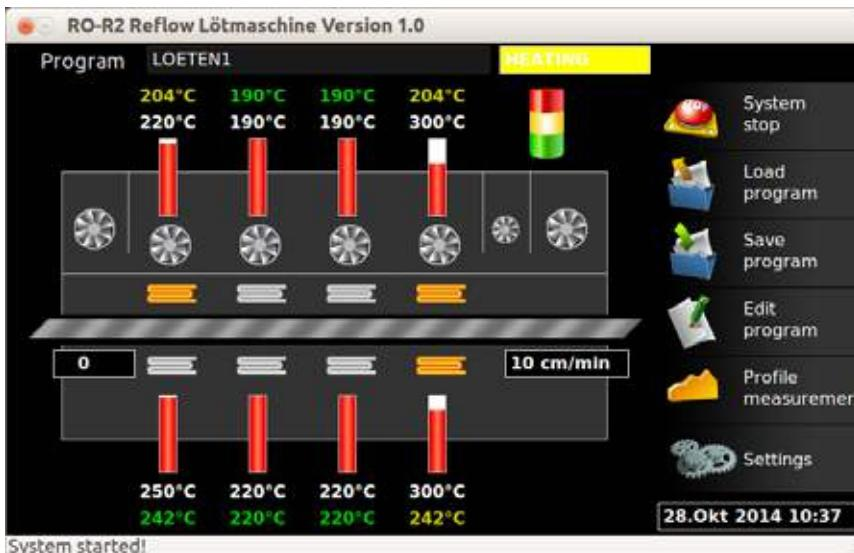
The soldering system will need approx. 15 - 20 min heat-up phase to heat-up the oven from room temperature to operating temperature for the soldering process and to reach ready state.
