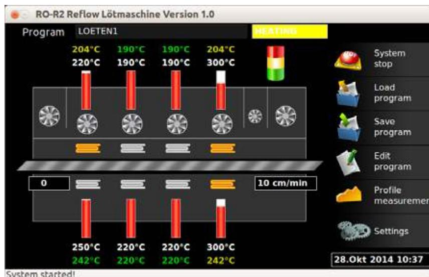
By stopping the system the heating will be switched off. The fans and the conveyor are still running to avoid a heat accumulation and an unequal warming of the drive. The operating status is changing from READY to COOLING and is shown in the status message of the system screen.
