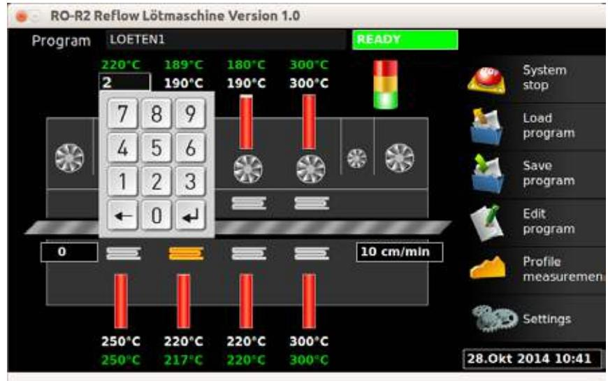
When tipping on the selected nominal value its display will change to an input field and a virtual keypad will be shown on the touch panel.
