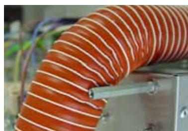
The distance bolt is used as a guidance for the exhaust hose. The hose must not be placed on the distance bolt.
