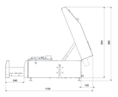
All dimensions in millimeter (mm)
