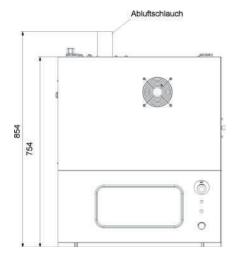
Dimensions of the soldering system with opened hood
