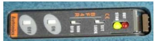
**2. Dark On Mode:** 1) If you want to detect and count the space between parts, press”ON”
