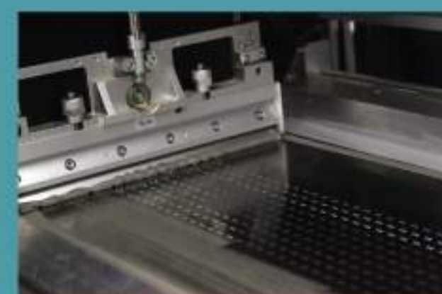
Custom design clamping device that helps to hold long PCB straight and suppresses soft board bending problem.
