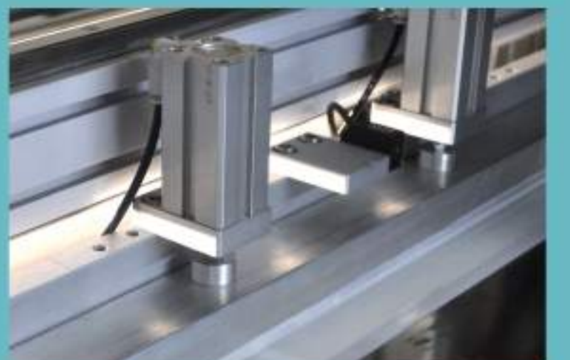
Highly adaptable stencil frame clamping system
