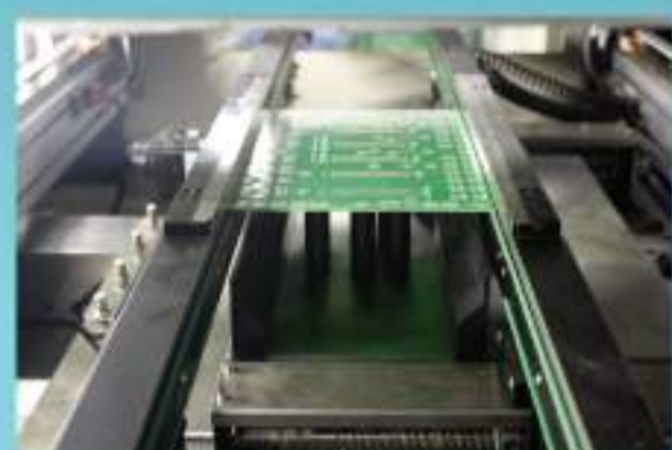
Advance clamping device helps to suppress soft board bending problem.
