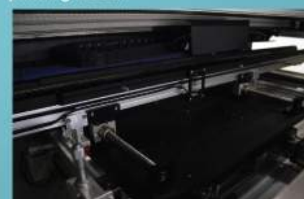
Accurate vertical adjustments of stencil frame driven by ball-screw in fast and quiet movements.
