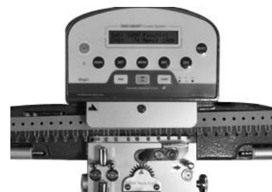
③ Radial device counting Lead the parts through the center sensor from left to right. Pitch value is -2.
