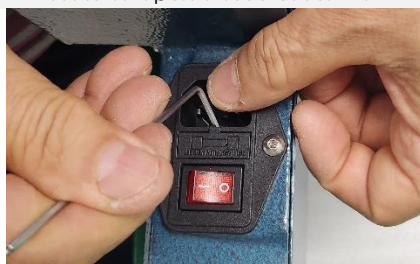
How to open a fuse cover - 1
