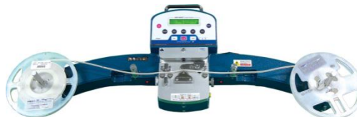
Giga S_ Automatic SMD Parts Counter including Pocket Check feature
