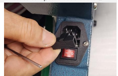
How to open a fuse cover-2
