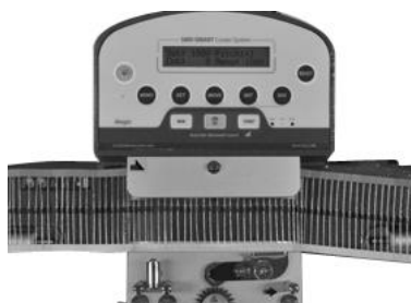
② Axial device counting Lead the parts through the center sensor from left to right. Pitch value is +1.
