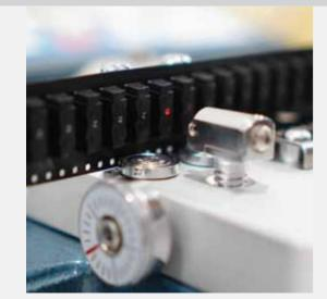
Easy adjustment the height of pocket sensor 8,12,16,24~48mm
