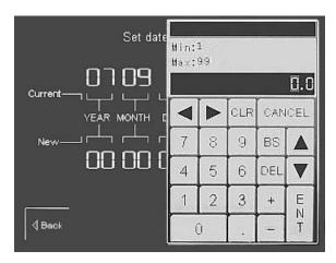
With the soft keypad appearing in the screen any number between 1 and 99 can be entered. Note that any number exceeding the maximum allowed value for the specific field entered will not be stored.
