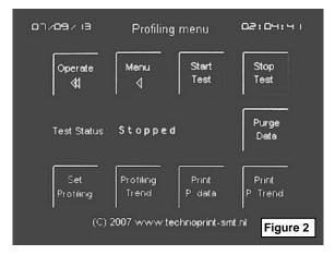
From this menu all options in the profiling software can be accessed. For that purpose this screen will be indicated as "Figure 2" for further use in this manual, when referred to this screen.
