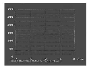
A screen like this will appear with graphs steadily changing for each temperature zone. When a thermocouple is connected a dotted line will appear indicating the probe's temperature.
