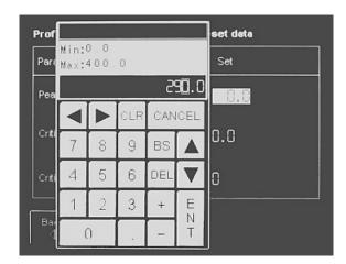
Either of these parameters can be entered by tapping on digits next to the variable. A soft keypad will appear and a value within the range indicated in the top left of the soft keypad can be entered.
