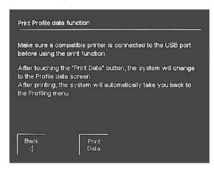
From the Profile menu(see figure 2 on page 11) the data captured as described in chapter 3.6.1 can be printed out to a printer connected to the USB connector located on the left side of the screen(see 5 appendix on page 21).
