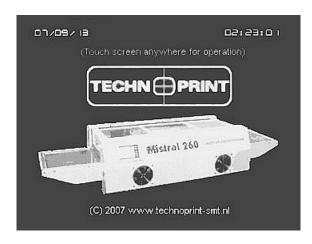
After the machine is started up with the main switch, the display will start automatically and you will see a screen that similar to the one shown on the left.
