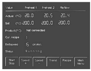
In the operator menu tap on the start the machine. The status indicator will display "Running" as shown in the screen to the left. When the machine has reached the desired temperature one can start a test run to collect data for printing or external storage. This is done by returning to the main menu.
