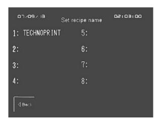
As an example under recipe number 1 is the name "TECHNOPRINT" stored. This name will appear in the operating menu when recipe number 1 is called up(see chapter 3.3). All settings entered with the soft keypad will be saved after powering down the machine.
