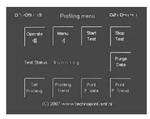
Now a profile can be made and stored for later use or referring purposes. With the thermo coupler attached to the PCB and the desired parameters entered, a test run can be made while the PCB is going through the process chambers.
