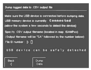
Collected data from the profiler menu can be "dumped" to a external storage device connected to the USB connector located on the left side of the screen(see appendix on page 21). To enter this option from the Main menu(figure 1 on page 11) tap on the bump button to open the screen on the left.
