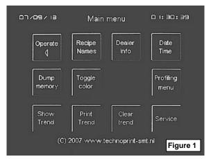
From here there profiler menu can be called up by tapping on the Profiling button in the main menu.
