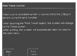
The temperature curve for each zone can be printed to a USB compatible printer when connected to the USB connector located on the left side of the screen(see appendix on page 21).
