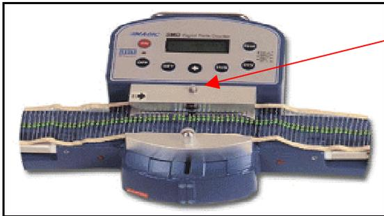
You can mark the tape with **Tape Marker** after the preset number is reached.
