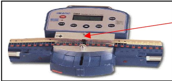
You can mark the tape with **Tape Marker** after the preset number is reached.
