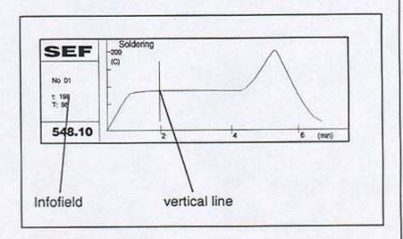
You can move this vertical line in the recorded procress curve. In the Infofield you will get in dependence of the vertical line the temperature and the time value.
